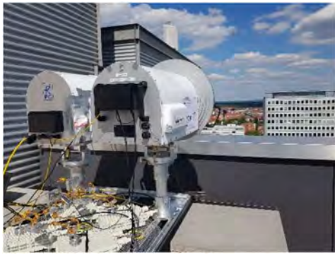
FIGURE 15. 300 GHz ThorLink connecting two buildings at the campus of TU Braunschweig.
